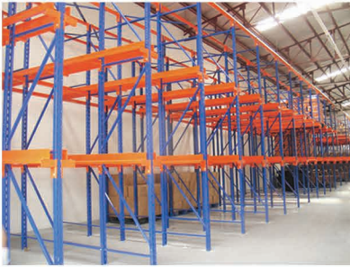
DRIVE-IN RACKING SYSTEM
